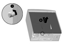
removing the pc access panel on the S0000 series model
